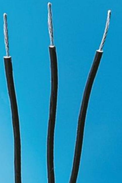
→ Project Success : New **antistatic wires** prototypes developed in target range ( $\rho \approx 10^8 - 10^{14} \text{ ohm.cm}$ )
